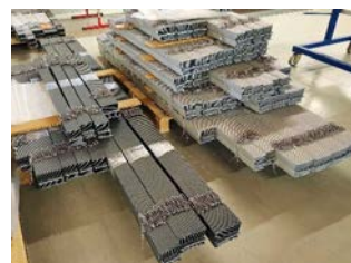
Uniform stack formation plays a key role in the fully assembled slat packs.
