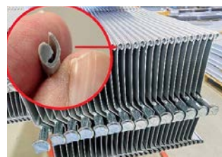
A plastic profile is rolled into the outer edge of the aluminium slats to protect against rattling noises and paint damage.
